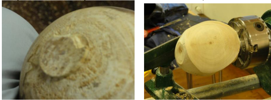
First bowl showing the failure Second bowl being shaped up of the foot.
