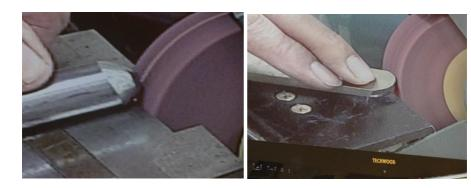
Using a platform the angle of which can be adjusted. It allows you to swing easily through the grind.
