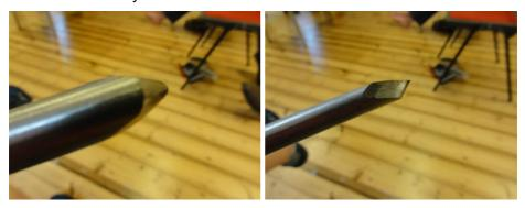
The finished spindle gouge with clean cutting edge.
