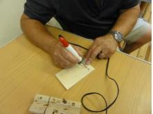
This 'pen' has a transformer and a form of temperature control.
