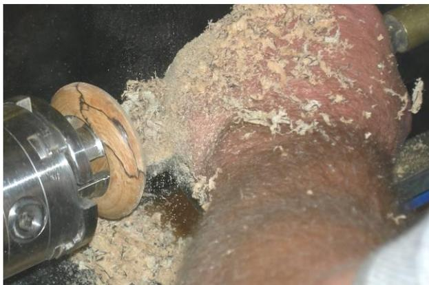
Having done the front face, it's sanded and treated, then reversed in the chuck and the back of the watch completed.
