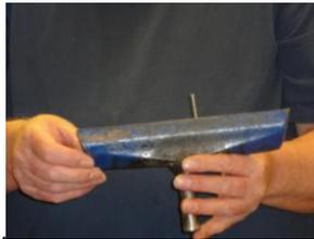
support, home made using a metal pin dropped into the support. This will stop your chisel being thrown outwards so ruining the edge of the wooden bowl.
