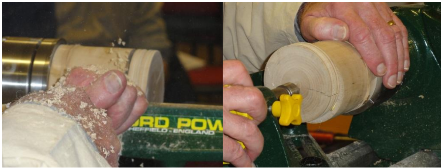
The jig being parted off main block Note the grooves for elastic bands
