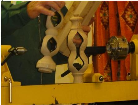
Start with four identical pieces which have been 'paper glued' together.
