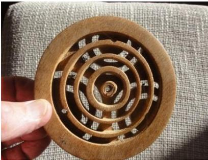
First a tea pot stand using a parting tool to cut the grooves and offset the circles on the underside. Just cut half way through.
