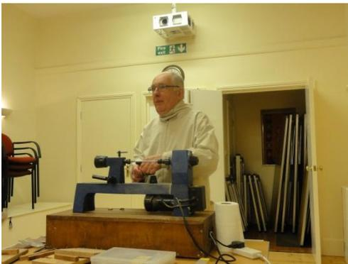
So starting with the blanks these need to be drilled out fitted onto the mandrel and turned down to the desired size. If you are using a plastic blank it pays to warm it first other wise the drilling may shatter the plastic. This is because you are turning down to a very thin tube.
