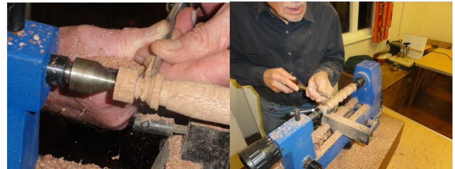
Parting tool used to round off end. A variation.
