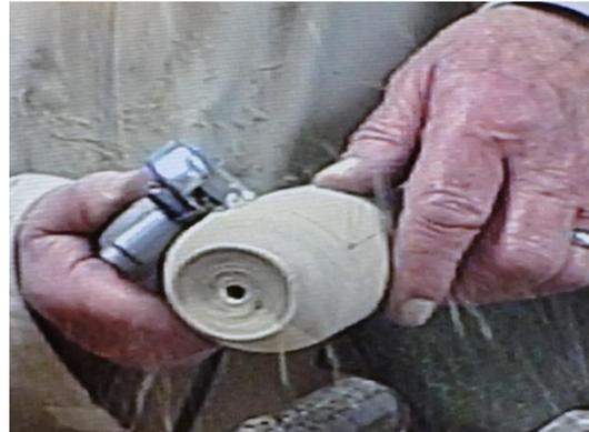
Slot cutting tool and actually making the cut
