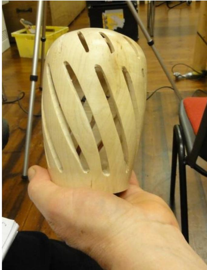
But first you have to shape up the piece so it will look fine in the finished form. Ken suggested that a simple vase shape allows for easy cutting of the slots since you work on a convex surface when making the slots. Also
