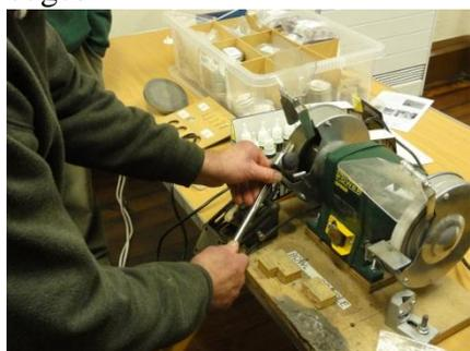
Ken's other machine is a basic grinding wheel but fitted with a white wheel and a CBN wheel. This latter wheel should last a life time(- say the adverts). Ken uses a Robert Sorbey gig to demonstrate sharpening a bowl gouge. Other firms offer similar gigs that allow you to roll the chisel across the grinding wheel. Note how stand has marks for setting up each toll to get the right edge.
