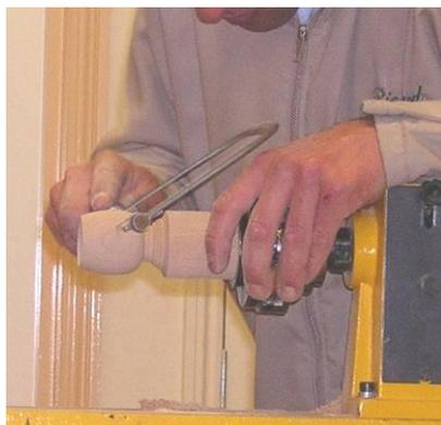
Once you're happy, cut out the section of the bowl using a coping saw, or similar. Then it's onto the handle. This is just a basic big flattish cove. Work down from both sides, down to the centre of the cove, then round off the end, leaving enough wood to be substantial enough to allow you to sand off the handle before you
