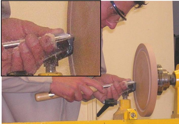
Now to the cutting in of the cove on the front face. This is of course optional, but adds a bit of decoration in what would otherwise be a glorified round plank, and will catch meat juices if you're making a carving board. I never much fancy using wood as a medium for carving meat on, but I suppose I am weird. Anyway, the cove...
