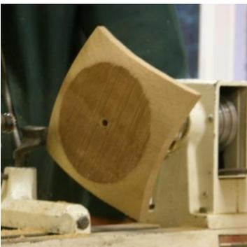
As the bowl got deeper, he left an 'island' in the centre to give it stability, and cut the top first. He kept stopping to check the thickness with callipers (the bowl thickness should be the same as the wings).
