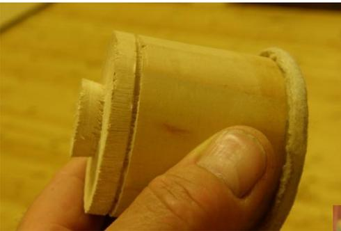
He then cleaned up the foot, by giving it a small dovetail shape using a 3/8" spindle gouge. He also reduced the thickness and
