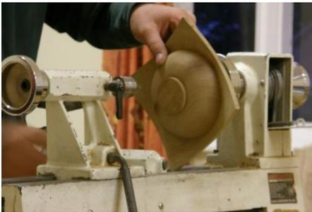
Next he needed to turn the work around again to finish the foot. For this he used a specially turned piece of wood with a felt pad glued to it. This was mounted in the chuck, and then the bowl placed over it and the tailstock secured it in place.
