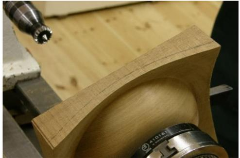
frequently to adjust the rest and also to check on the thickness of the wings (and to make sure the thickness is consistent from middle to edge). Another aside here where he mentioned that he prefers Ashley Isles chisels as they seem to keep their edge longer.
