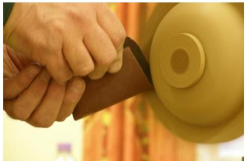
save time). Slow the lathe down to 700 otherwise you might overheat the work. He used a sanding pad for the wings, and finished them off (sanding with the grain) by hand. If the end grain is a bit rough you can lightly spray with water to lift the grain and sand again after letting it dry out.
