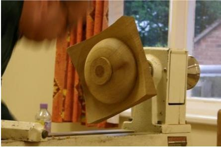
to the work to give the gouge plenty of support, but always stop the lathe first – in fact you need to keep stopping to check the shape anyway.
