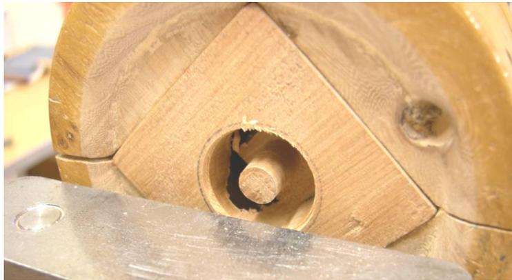
Once the hollowing out of the surrounding area is complete, a plug is fitted into the 30mm bore surface, which will serve to locate and secure the tip of the star into centre of that face of the workpiece. The plugs have a 2.5mm hole in the centre to locate on
