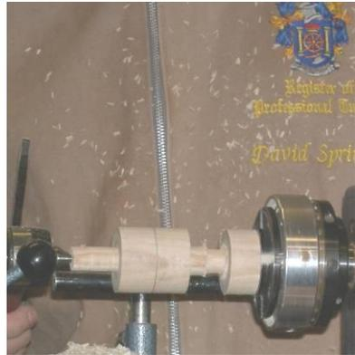
If you turn down the end diameters accurately in the zone which will be the waste wood, then you can more reliably and quickly get the non-waste section to size. Once the 15 mm diameter has been produced, and the centre section of the cone produced, (the solid lines below) it's just a matter of continuing along the (dotted) line at the same angle to produce the cone.
