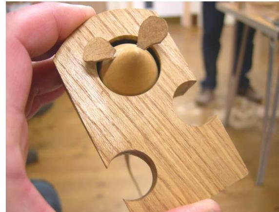
The mouse is a teardrop shape and is a push-fit into the hole in the cheese. The hole is hollowed out a bit on the inside so that the mouse's backside drops into the hollowed section, which then makes it poke out of the hole at an angle, so it's not going to fall out.
