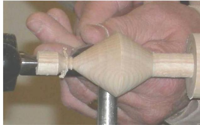
Once the first point is done, again follow the line of the other slope, to part it off with the skew chisel, working back toward the chuck, and taking out the waste wood as you go, to allow access to the skew.
