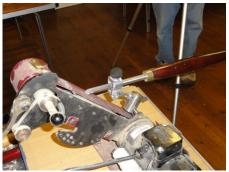
In the left picture we have a skew chisel and on the right a spindle gouge being sharpened. Note in the right picture how the chisel is held in the jig and rotates over the grinding belt.
