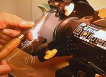
Using a spindle gouge to demonstrate Mick first grinds the end to the correct angle (left picture above) then rolls the end gently over to give it an edge(right hand photo). With practice Mick says confidence builds and it certainly is a very quick method. Various firms make jigs to help get the angle correct. The jigs allow you to swing the gouge across the
