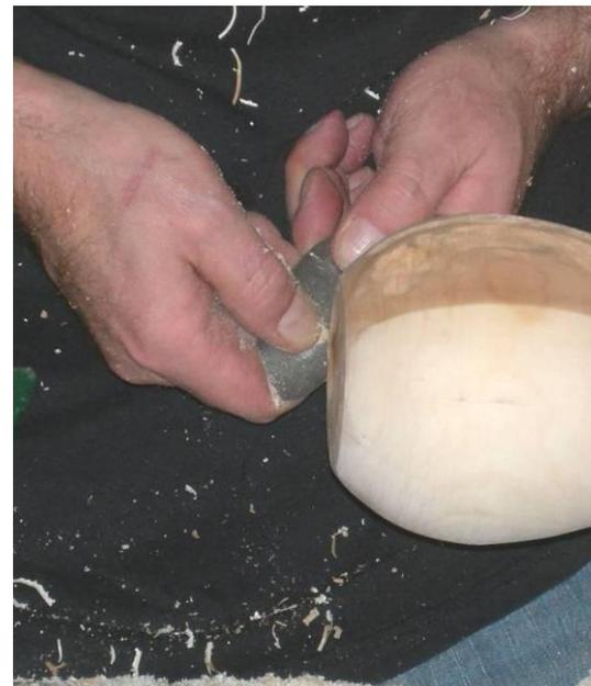
Another cunning device to make shapes flow nicely together is the cabinet scraper. Put a burr on it by running it across a grinding wheel with the tool rest horizontal. Use the scraper on the lathe without a tool rest and have it trailing the direction of cut at 30-45°. You can buy cabinet scrapers from most hardware outlets, they are generally less than a tenner.
