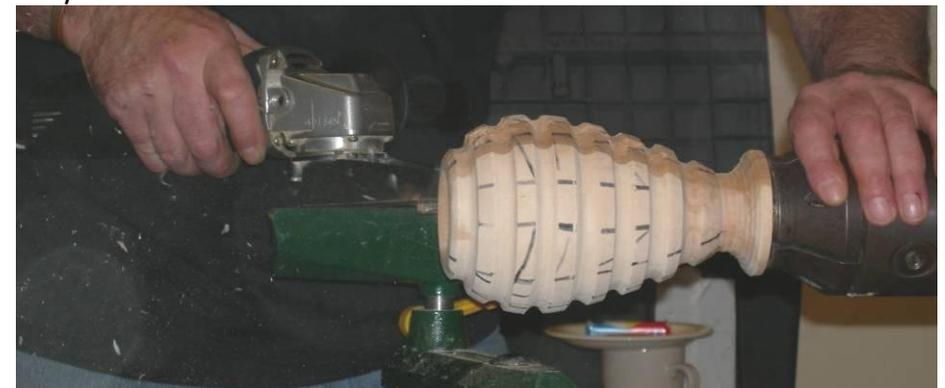
It's not very clear in the picture above but the tool is supported on the tool rest while it's moving across the work. Mark had to hold onto the chuck on our lathe to stop it from turning, which is obviously not ideal, the shaft should be locked if possible.
