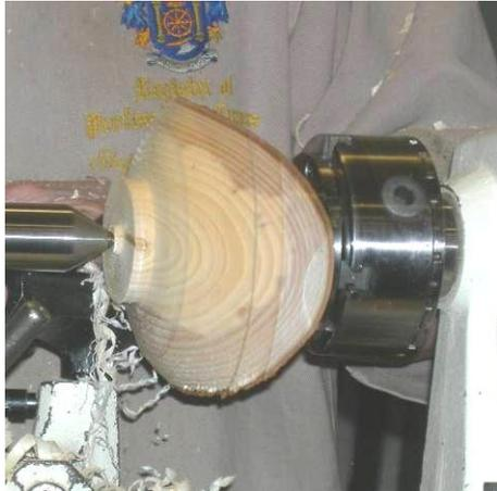
Turn the base spigot and the outer walls of the bowl before reversing it in the chuck.
