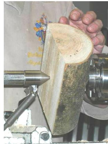
The tailstock centre was used to help support it to start with.
