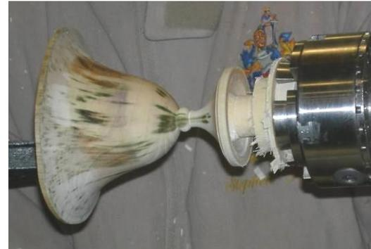
Steve then demonstrated turning a thin walled vase. This wasn't with green wood. He started by doing the inside, turning it to as good a finish as possible. Once the wood fully dries out and moves around you won't get a second chance
