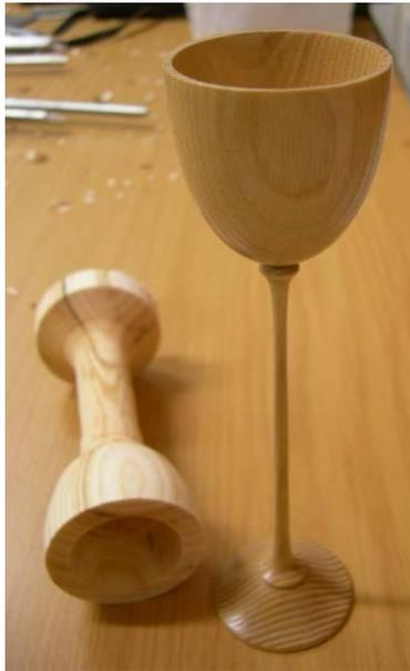
Once the bowl is done, rough the stem of the goblet to about the same thickness and the right kind of length, and leave the foot with a spigot on. That's the turning done, the end grain is now sealed up with PVA glue so that the moisture in the wood has an escape route other than through the end grain, I guess so that it dries less quickly.
