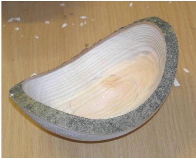
When finishing off the outside of the bowl, you can make a pad to fit in the chuck for the bowl to push on. Any marks made by doing this can be removed when you
