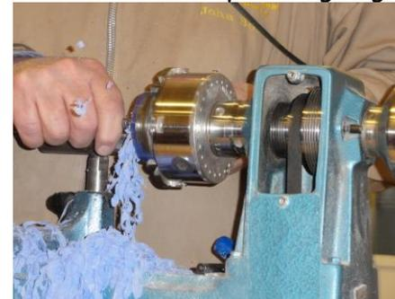
*John working on the box lid, hollowing out prior to using the unichaser tool.*
