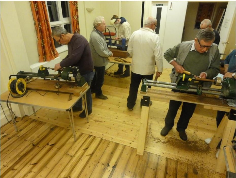
*How good are you with skew chisel? Members practising making a tapering dibber from square block using only a skew.*
