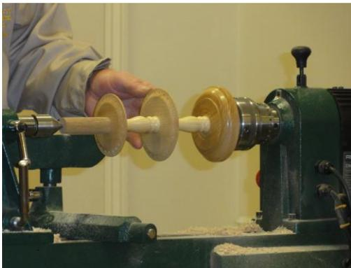
With the basic pillar and disks assembled it is now time to turn to the finial. This will top out the whole job so as John says needs to be distinctive. This can best be achieved by using a different and contrasting wood to the rest of the design. You can also use it for storing rings so it should come to a point.
