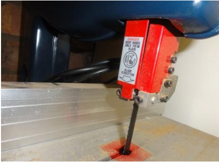
Different machine but shows array guide screws to adjust
