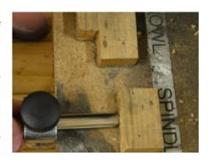
But back to sharpening.. Ken Croft brought along an Axminster kit which swings the tools round so you get an even clean edge on any hollow curved chisel. But as Ken pointed out you do need to set it up correctly. He had a set of stop marks actually screwed onto the grinding wheel base (picture above). There was also the water wheel cooled system which Roy demoed.
