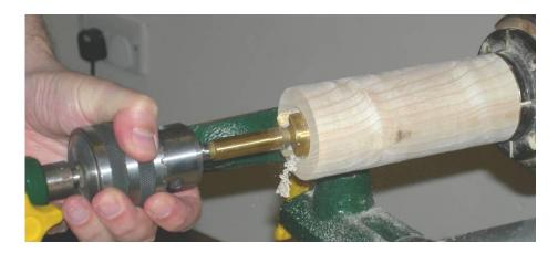
Then mark out the high and low points on the profile, and also the diameter at the outer end of the napkin-to-be. Then start profiling.
