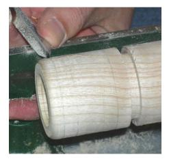
This particular napkin rings will have a pair of narrow grooves on the raised sections to let in a row of beads on each. The beads are glued into position using superglue. Each length of beads is cut one bead too long, as they will be scrunched up as they are glued on.
