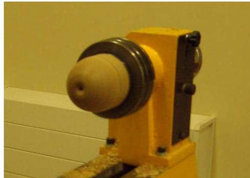
**Screw Chuck**, a piece of paper was placed at the back of the screw chuck to protect the finish. Cutting from the pencil line he rolled the gouge bringing up the handle at the end. Then going deep in the end from the centre outwards Richard performed a flowing curve blending both cuts using the bottom edge of the gouge to the finished shape the next stage was finishing as before.
