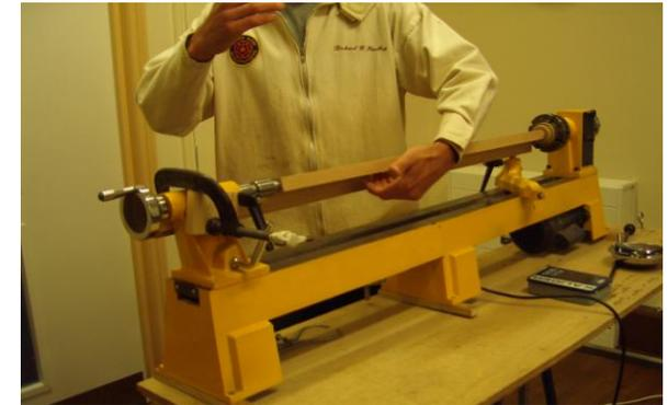
The problem of whip was overcome by using the right hand over the back of the "stick" as a steady, with the thumb holding the roughing gouge firmly down on the tool rest.
