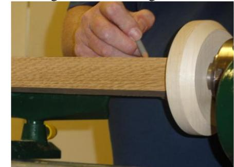
Mark out a pattern stick with each end of the curves on the master. Mick uses a skew to make the initial cuts. If you are going to have square ends then these need to be made first and delicately. Note in the right hand picture above the chuck being used has a square hole in the wood block with a screw plate attaching it to the actual chuck.
