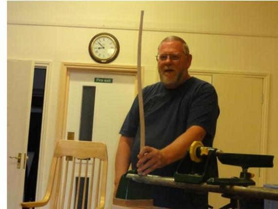
Mick outlined the construction and difficulties he had with making the chair but the hardest part were the shaped long dowels to the chair back. These are tapered and bent.
