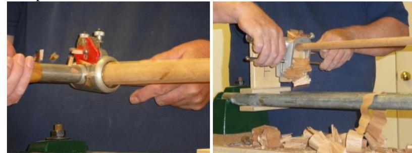
Whilst these back support stems can be turned; as you would a walking stick say, it is far easier to use a special tool. This is rather like a spoke shave which you push along the wood. There are several sizes which allow you to gradually reduce the diameter.
