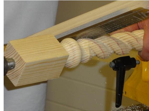
In the picture the larger microplane is being used to ease over the curves. You could use a Surform, both the flat and curved versions, but Richard felt these had too big a cutting face and tended to rip rather than shape the piece.
