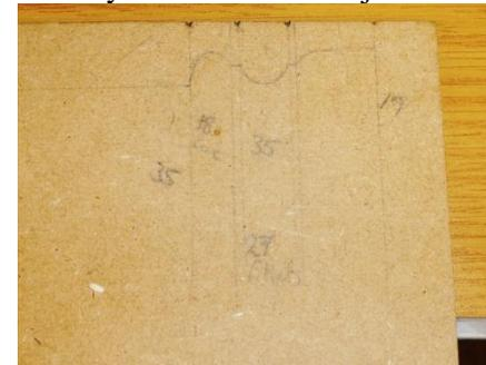
Making the first cut from the square end is important. Hold the chisel so it cuts away and into the waste. Make a start on the first cove next to the square end. Then you can round off the whole section to give the roughly tapered section you are going to work on. Now use your template to mark up where each cove
