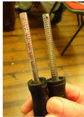
The red line is now cut down using a small saw. In effect you are transferring the line to a lower position. Now widen the cut using a microplane. These come in various sizes. You can obtain them from Axminster. Once you have a decent cut you can shape it up so it rolls over the peaks and troughs. For this you can use a larger microplane and a sanding strip.
