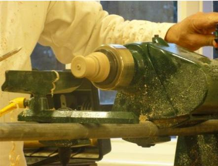
What Nick demonstrated was to turn a simple bobbin with a central hole through the middle. The two edges or rims needed to be serrated. Leaving them smooth would mean the 'tank' just skidded on one spot.
