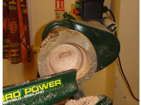
Glen Teagle made the hollowing tool Nick used on the night. It shapes by cutting very narrow ribbons. When the edge of the cutter gets blunt you just move it round a fraction. There are many similar hollowing tools on the market.
