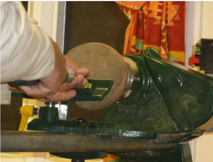
With the inside work it pays to drill out to the final depth first. You can do this as shown above with a spindle gouge using it more or less as a drill.
