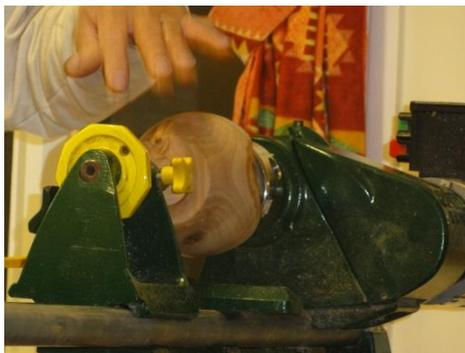
Nick was using a screw chuck which on this occasion took two of us to release it. Also note that care needs to be taken when stripping off the bark as this has a tendency to come off in chunks.
