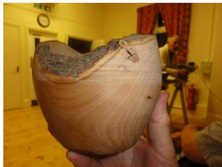
The final shape although still to be finished off and a bottom flat put on it.
