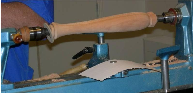
Notice that by using a piece of laminated paper as a background, you can see subtleties of the turned profile more easily. It's useful to have some Rare earth magnets around for sticking things like this into place too. Axminster.co.uk sell the magnets in packs of 10 for about £5.50.
