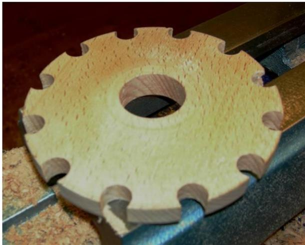
Now for the actual necklace holding bit. This is basically a disk with a series of holes on the outer edge, which break into the outer edge.
