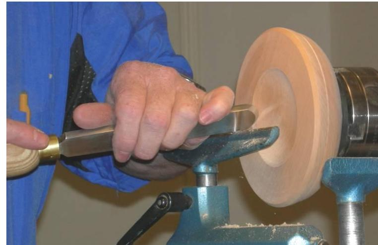
The base was then put back on again, clamping on the inside of where the spindle will fit. Remove the area previously used to hold the workpiece, so that it's not obvious how it was held.
