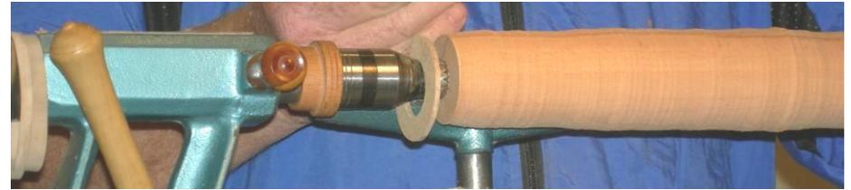
Having turned the taper put a small bead between the taper and the rest of the workpiece. This ensures that surplus glue that runs out of the joint will be hidden from view.
