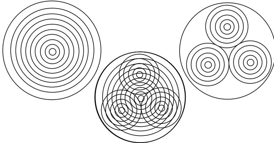
The object of the demonstration was to produce in a 6mm thick disc, a series of concentric rings 3mm thick, 3mm deep on one side, then on the other side to produce three sets of concentric rings with centres differently placed from the original rings, also 3mm deep, such that the rings would break through into one another so that in places you could see from one side through to the other.
