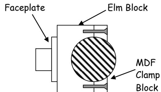
This will allow the sphere to be locked into position for turning each point in turn. Clamp in the sphere with the North or South pole facing exactly outwards, using the tailstock to ensure its exactly in place.
