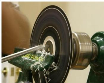
Then he took the middle out. When hollowing out you need to use a smooth movement and try not to leave a pimple in the middle: swing round until the tool touches your belly (and this may be sooner rather than later for some) and then move your body in to finish with the tool in the middle of the bowl. Listen to the
