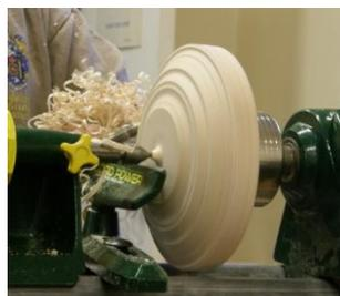
Once the bottom is trued up, create a chucking point and then refine the profile and soften the curves to make a natural transition. Then remove the spigot where the tailstock centre was, and re-make the centre hole for later use.
