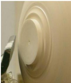
Now dovetail the chucking point, making the base around it slightly concave, which will help in centring the work on the chuck. It is important to get the diameter of the chucking point as close as possible to the optimum diameter of the chuck (that is, where the jaws form a perfect circle) – this will also help to centre the work on the chuck and will also reduce the amount of marking the jaws make on the wood.
