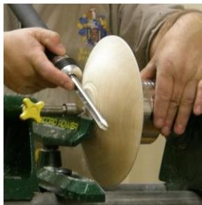
Put the toolrest up against the centre and using a bowl gouge take off the chucking point, leaving a slightly concave base.
