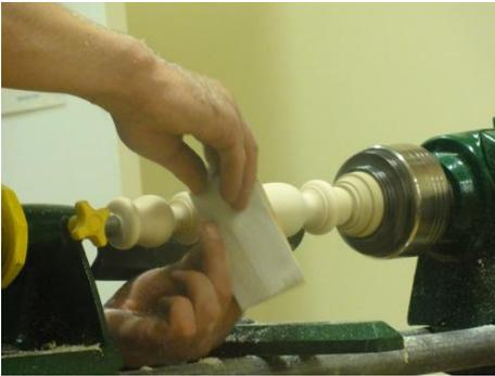
At this stage do not curve the shape just cut to the critical dimensions so you have the necks in the right place and right diameter. Richard used his skew chisel to shape up the stem but he felt most members would use a spindle gouge. He recommended cutting the beads first then the coves. This usually gives a better result.
