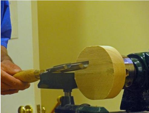
*Roughing out chisels and starting block*
