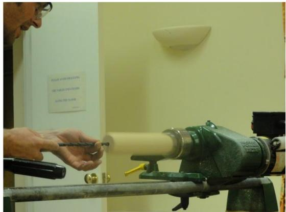
*Drilling out hole in stem*
