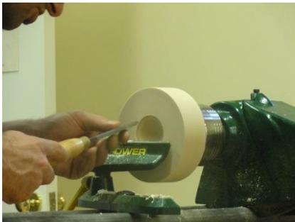
*Hollowing out for cable loop*
