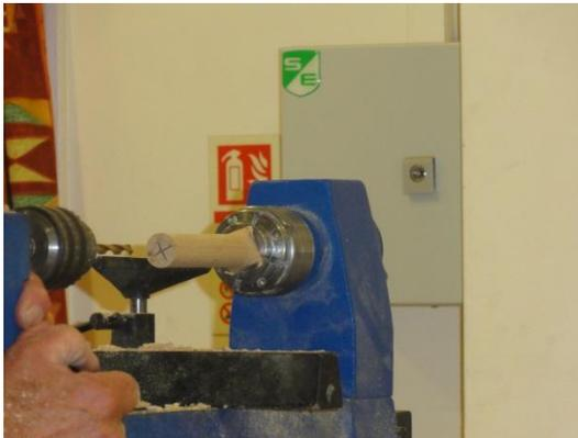
Start with what is really a very thick dowel about 8cm long. Drill out a hole for an insert which will come from a say 7mm diam. dowel. This will be your hook.
