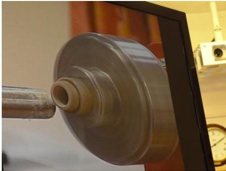
The bottom of the box now has a matching spigot end. Remember the thread work will reduce the diam. further. This time the thread will be made using the bottom edge of the chaser. Again apply at a slight angle to get that initial cut, then let the tool do its
