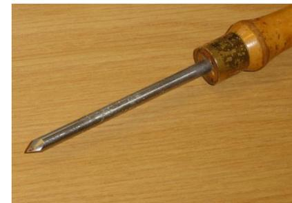
Tools for this small scale work were a small point tool and a round scraper with a bevel cut on the very end. Plus, very important in John's view, an arm rest to help the delicate control of the tools. Plus, of course, a thread chaser. A universal chaser has the top face for one thread and the bottom for the matching thread on the matching part.
