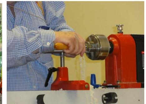
As John pointed out anything faster and it would be difficult to create a thread. The resin blank offered several advantages in that its dust was heavier than wood and also none allergenic.
