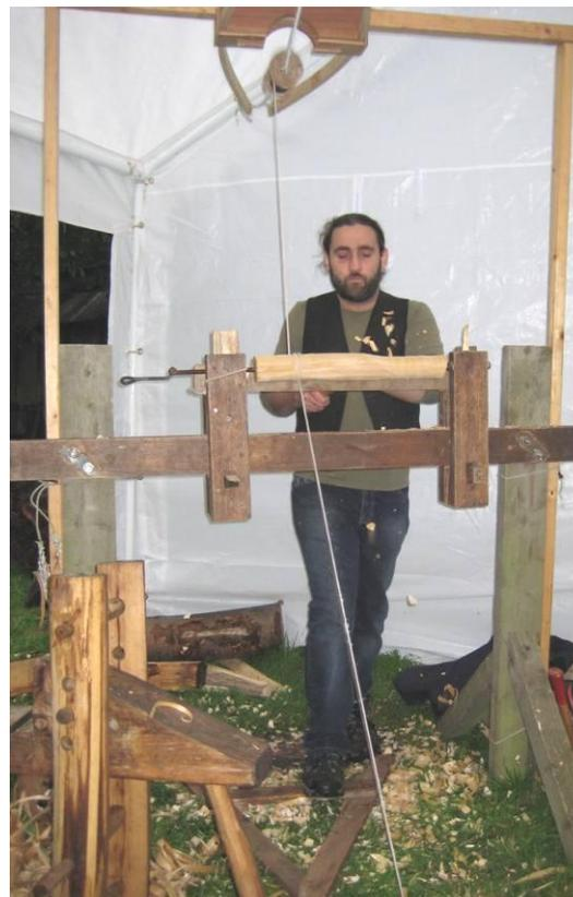
As a demonstration Matt very quickly turned a piece of ash into "ye olde rounders batte" - that's pole lathe marketing speak - and achieved a very smooth finish straight off the skew chisel. (Calling things "olde English ..." also works well apparently! )
