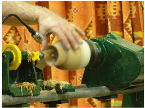
The aim, of course, is to match the outer curve of the main bowl through the underside. The splayed hollow cylinder will be the legs after cutting. It is advisable to go for three legs as these will always 'sit'. Four might look better but the finished bowl usually has a wobble.
