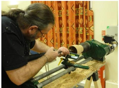
Mark switched to a hollowing out tool - a 'munroe'. Work down in stages so you can check the wall thickness. Check that the wall thickness is consistent, as this can avoid splitting as the wood dries out. In our demo it did split and had to be wrapped with masking tape. This hiccup meant that support for the next stage might be a bit dodgy. So Mark used a golf ball to give that bit of extra help in holding the bowl whilst the inside is cut away.
