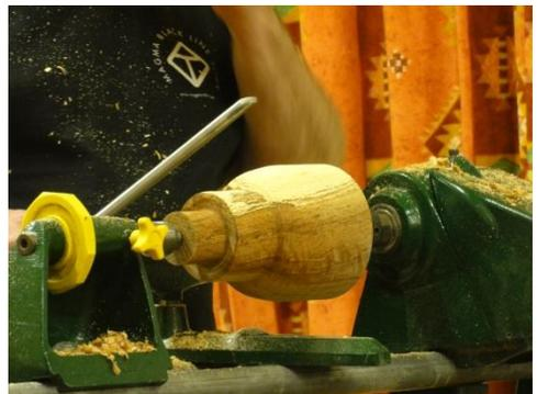
Mark started with a freshly cut log of oak. Using a ring centre, to ensure a good grip, the log was rough turned into a cup and stand shape. Mark used a spindle roughing out gouge to get down to a near finished shape.
