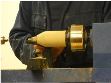
Using a parting tool to cut the rings
