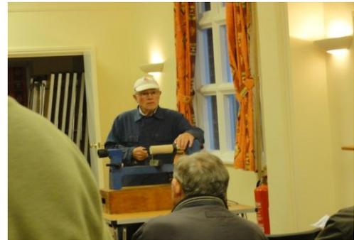
Make the cone shape first and there is no need to sand. In fact the slightly rough texture adds to the appearance. Then drill a fine hole in the apex for the hanging string. It is best if you do this with the lathe as it tends to get difficult if you try drilling using a hand drill.
